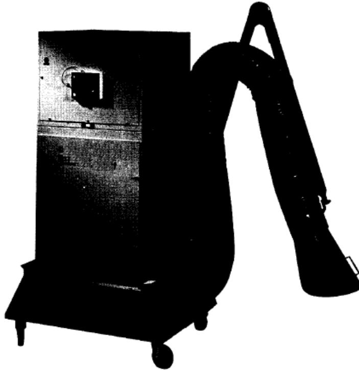
*The M66 is a self-contained media air cleaning system designed for use in source capture applications where mobility is desired. The M66 can be ordered in a three-stage filtration which will effectively remove a broad range of airborne contaminants including fine dust, smoke, soot, vapors, mist, VOC's and more at a rate of up to 2700 cfm.*
